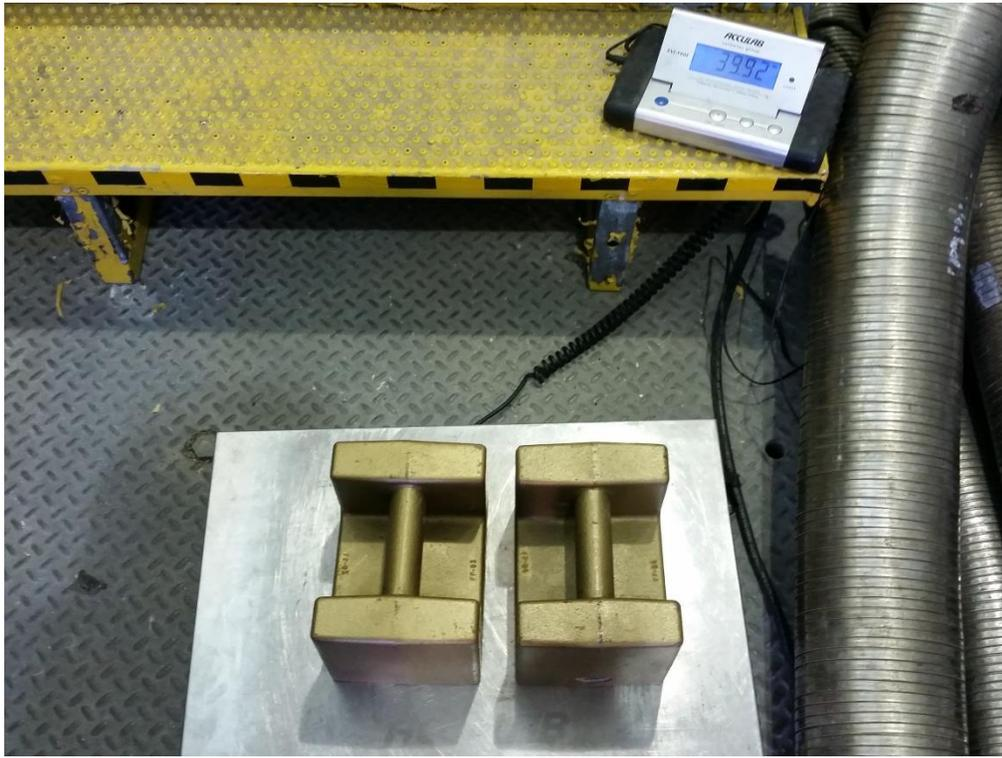
Figure 10. Scale verification using calibration weights
