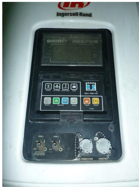
Figure 6. Temperature control for the refrigeration unit
