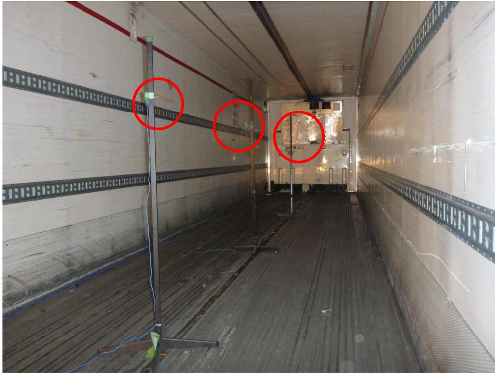
**Figure 12. Position of the three thermocouples in the middle of the trailer**
